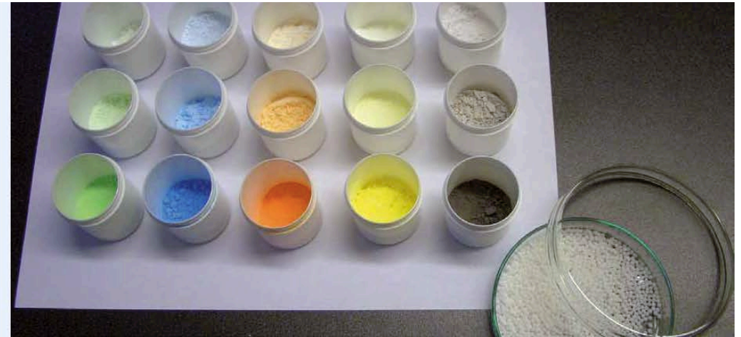
Trituration of colour pigments with lactose in steps of C1, C2, C3 describing different concentrations in a dilution of 1:100.
